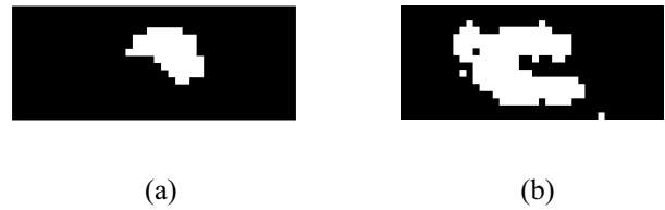
Fig. 4 16×40 proximity image of the user’s hand recorded from the multi-touch pad (a) Pinky side of the hand. (b) Partial palm.
