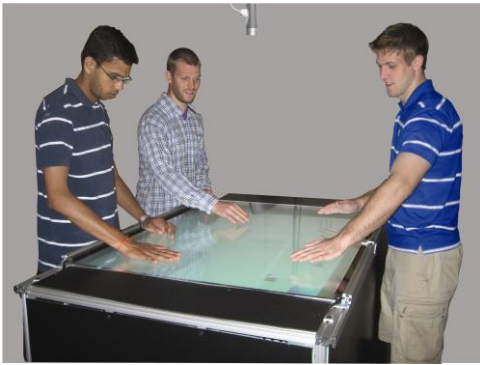
Figure 1: Three users working together using a rear-projection multi-touch tabletop display augmented with hand tracking using an overhead camera.
